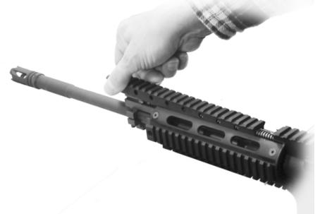
5. Retract the spring to release it off the spring clip, as shown. Push the spring clip back towards the spring and lift it upwards to remove it from the op-rod. It may necessary to gently tap the spring clip to release it.
