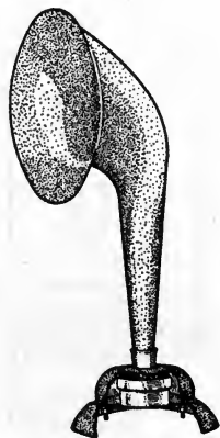
FIG. 50.—Horn type of loudspeaker.
