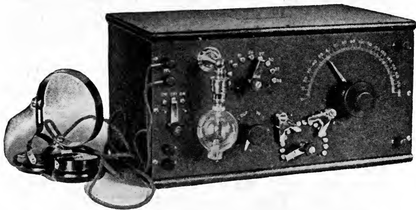
FIG. 33.—Radio receiver of 1913, comprising audion detector and contained tuning element, with dead-end switches.
