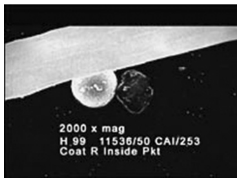
Figure 6.9 GSR particle from the evidence against Barry George in the Jill Dando case.
