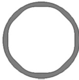
Figure 4.10 Conventional eight-groove rifling.
