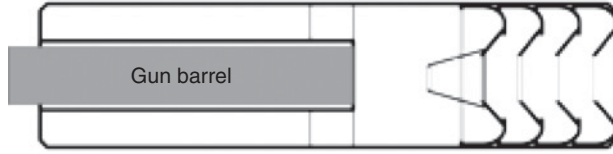
Figure 1.22 Typical silencer construction.
