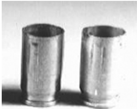
Figure 4.20 Scoop chamber marks on fired cartridge case.
