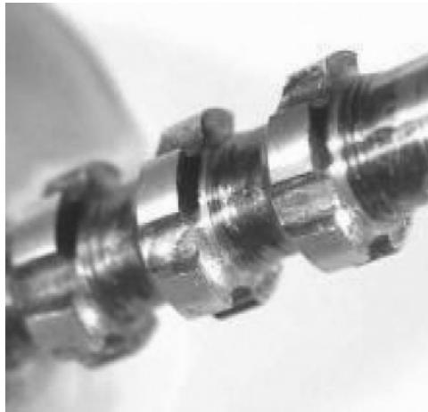
Figure 4.6 Broach rifling cutter.
