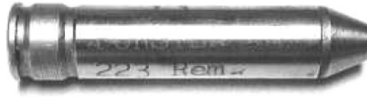
Figure 1.21 Rimless cartridge headspace gauge.
